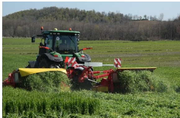
Yellow shield on the left catches mowed forage and drops it in a non-drying lump. Raising the shield on the right allows the forage to flow through unimpeded and fall in a loose porous uniform swath.
