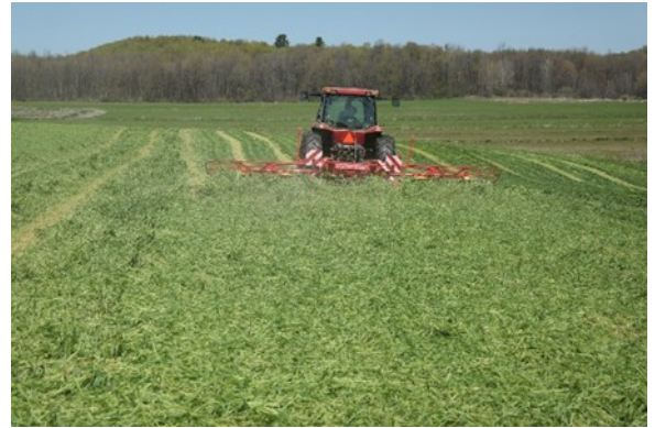
Tedders need to be operated at the design speed. Faster field speed will create non drying lumps.
