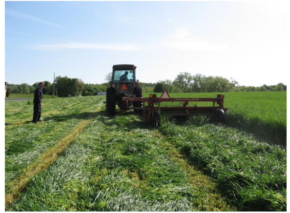
The left swath with the deflector down clearly shows the non-drying lumps it makes. On the right, the flow through wide swath is uniform and less dense to speed photosynthetic drying.
