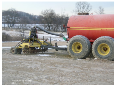
Mark Anderson attached an Aerway directly behind his manure tank for one pass incorporation. He since switch the drop tubes to the front of the unit as you can see in the picture below, it covered the manure and held the nitrogen more efficiently
