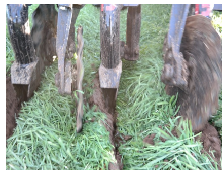
The coulters/injector handled a heavy winter forage sod, injecting 8,000 gal manure/acre.
