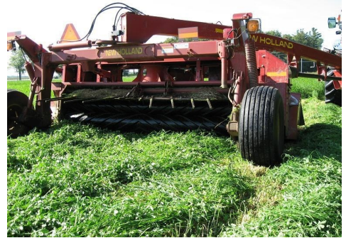
Bruce McCuaig, Lancaster, Ontario put his own spreaders on to increase his swath to full cutterbar width.
